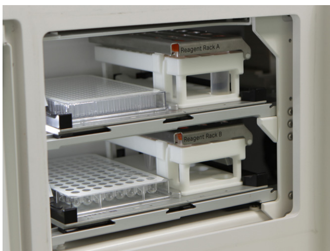
Fig 4. The sample hotel of Biacore 1K+ and Biacore 1S+ accommodates two trays. Each tray can hold one 96-well or 384-well plate and one reagent rack.
