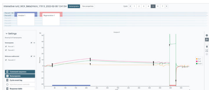
Fig 15. Example of an Interactive run . Each cycle contains an analyte injection (variable concentration) and a regeneration step. The full data set (seven cycles) was then fitted to a 1:1 model in Biacore Insight Evaluation Software (data not shown). (Analyte: beta-2-microglobulin. Ligand: Anti-beta-2-microglobulin amine coupled to Sensor Chip CM5).
