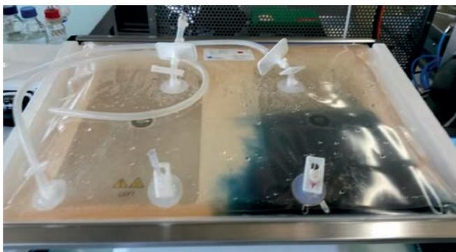
Fig 5. Illustration of the two separate compartments during de-colorization for determination of mixing time in the 20 L Cellbag culture chamber.
