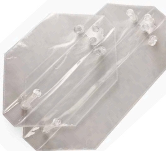
Fig 1. Flexible 3D plastic bags (empty) from the ReadyCircuit range similar to those used in this mixing study.
