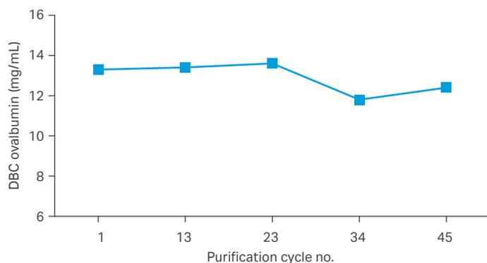
**Fig 8.** DBC of Capto Core 700 for ovalbumin measured over 45 purification cycles with 1 M NaOH in 27% 1-propanol as CIP agent. CIP protocol after every eleventh cycle was 5 CV CIP agent, 30 min pause, then 5 CV CIP agent. Fouling of the resin between DBC measurements was performed with MDCK cell lysate.
