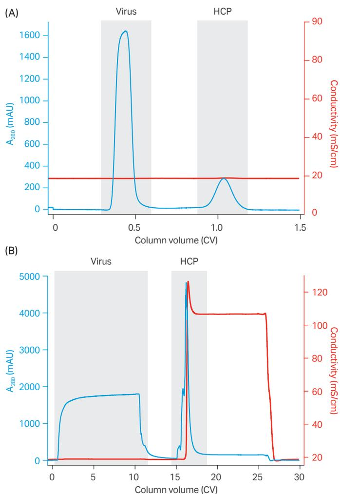
**Fig 3.** Chromatograms from the purification of influenza virus HA in the size range 80–120 nm and removal of HCP from virus material run on (A) the conventional SEC resin, Sepharose 4 Fast Flow and (B) Capto Core 700 resin.
