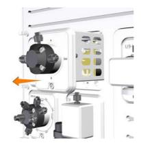
5 Disconnect the cable and secure it in the slit.
