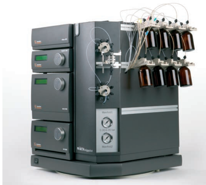
Fig 1. ÄKTA oligopilot 100 was used for the initial optimization and initial scale-up to 380 \mu mol.
