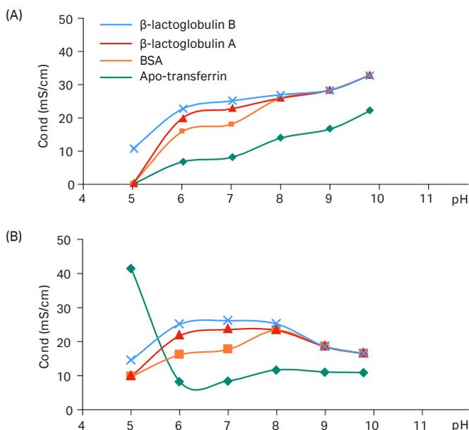
**Fig 9.** Elution conductivity as a function of pH for a set of model proteins on (A) Capto Q, where only the change in surface charge of the proteins influences the elution position (B) Capto DEAE, where both the change in surface charge of the proteins and the changed charge of the ligand determine the elution behavior.
