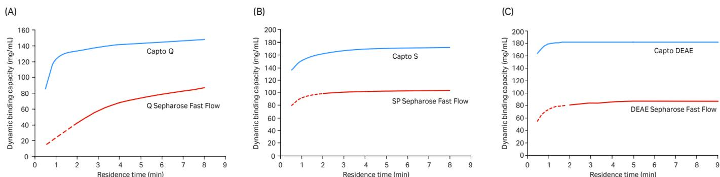
**Fig 3.** Dynamic binding capacity as a function of residence time for: (A) Capto Q and bovine serum albumin (BSA), (B) Capto S and α-chymotrypsin, (C) Capto DEAE and amyloglucosidase. For Sepharose Fast Flow resins, residence times below 2 min are not possible in large-scale columns.
