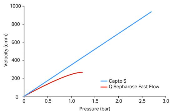
**Fig 2.** Pressure/flow curve for Capto S compared to Q Sepharose™ Fast Flow. Running conditions: AxiChrom™ 1000 for Capto S, Chromaflow™ 1000 for Q Sepharose Fast Flow, 20 cm packed bed, with water at 20°C. The pressure includes pressure drop from the bed and the column. System/tubing pressure is excluded.
