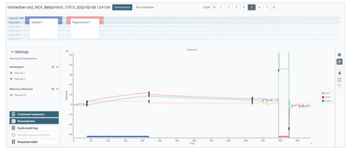
Fig 8. Example of an Interactive run . Each cycle contains an analyte injection (variable concentration) and a regeneration step. The full data set (seven was then fitted to a 1:1 model in Biacore Insight Evaluation Software (data not shown). Analyte: beta-2-microglobulin. Ligand: Anti-beta-2-microglobulin amine coupled to Sensor Chip CM5.
