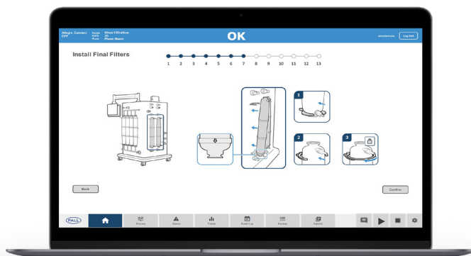
Fig 16. Guided instruction for installation (IFI), where the operator is instructed by the recipe to install virus filters.
