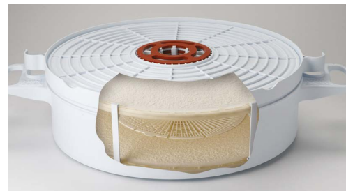
Fig 16. Cut away of a Stax CF module showing the internal volume for retained solids of up to 13.2 L per module.
