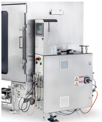
Fig 8. Electric cabinet attached to mixing tank, pictured with controller on top.
