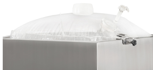
Fig 14. Fully inflated biocontainer extends above the top of the mixing tank.
