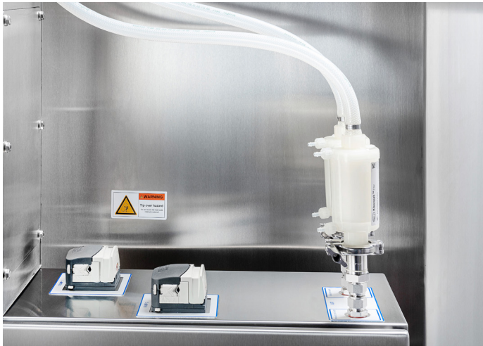
Fig 5. Inflation sets are used to connect the inflation system, which is found in the electrical cabinet, to the biocontainer.
