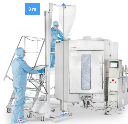
Fig 13. Minimum ceiling height required when using 3000 L mixing tank with 30 L powder bag and optional compact hook for powder lift.
