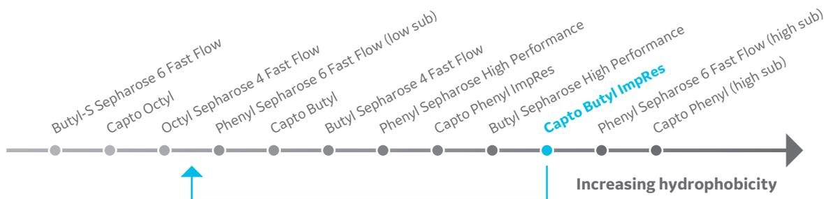
**Fig 2** Hydrophobicity scale with model proteins from data file 29031925AB. The arrow highlights how hydrophobicity differs for Capto Butyl ImpRes with the mAb compared to different model proteins.
