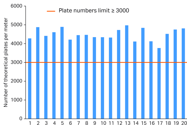
Fig 3. Efficiency analysis for 20 different MabSelect SuRe™ Validation columns showing high quality packing with theoretical plate numbers per meter above the limit (3000) and consistency between the packed columns.
