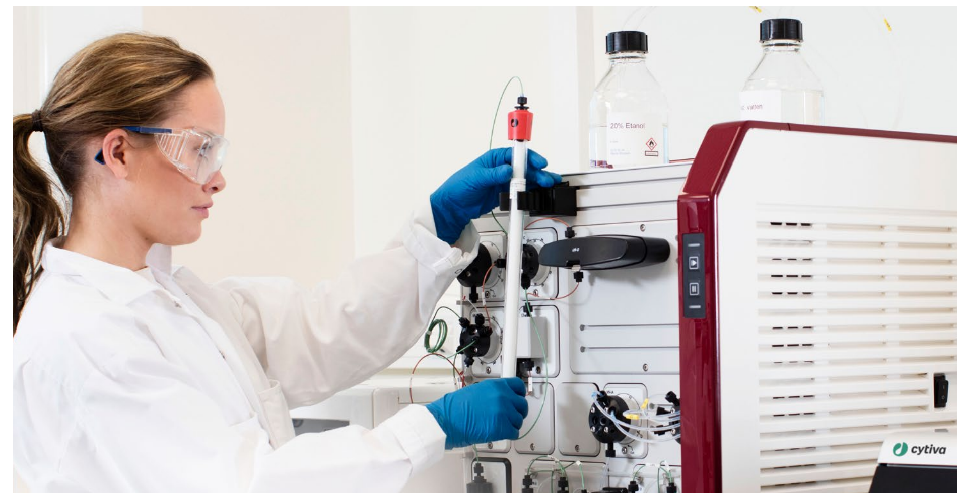
Superdex 200 Increase 10/300 GL column (10 × 300 mm) in use on an ÄKTA pure system.
