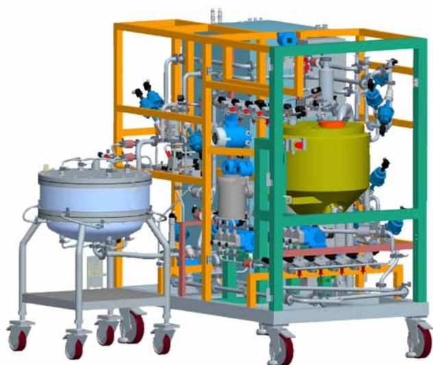
Fig 2. A schematic diagram of the SBIP BioProcess system, displaying the boiler reservoir (yellow), which is connected to the steel column (light blue-gray) outside the main frame of the system.
