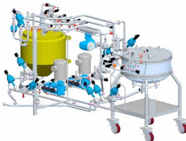
Fig 3. A schematic diagram of the flow system connecting the boiler reservoir (yellow) to the steel column (light blue-gray).
