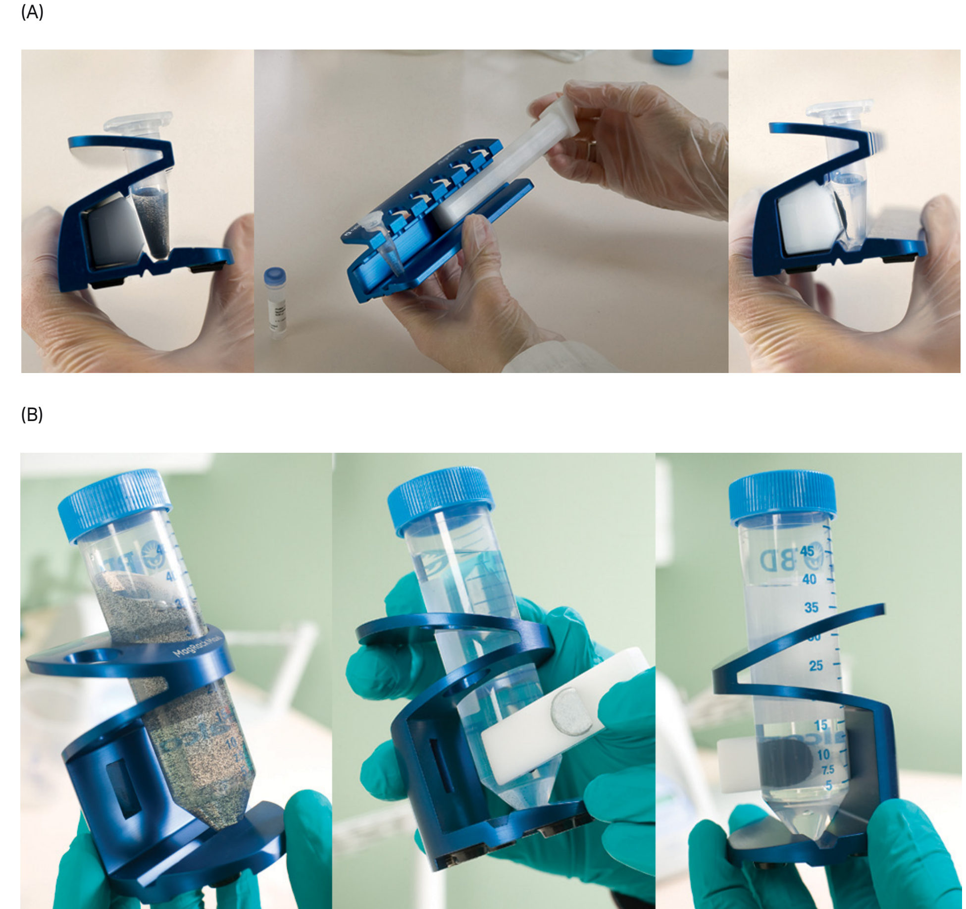
Fig 3.9. (A) MagRack 6 and (B) MagRack Maxi magnetic racks consist of an aluminum housing with a detachable magnetic bar. When the magnetic bar is inserted (center images), the high-density magnetic beads become attracted to the magnet in seconds. This allows easy removal of supernatant while the magnetic beads remain in the tube (images on the right).
