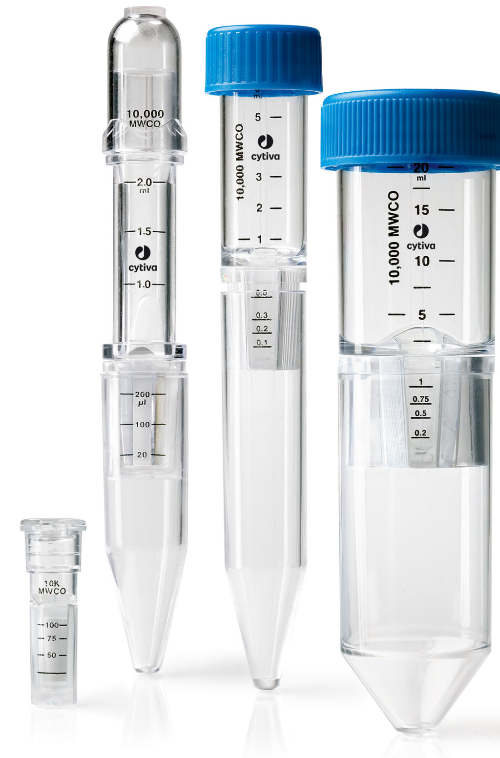
Fig 4.4. Vivaspin 500, 2, 6, and 20. All four products are available with MWCO values of 3000, 5000, 10 000, 30 000, 50 000, and 100 000.
