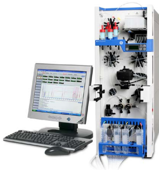
Fig 1. ÄKTExpress™ is a compact chromatography system supporting 28 different single- or multi-step protein purification protocols
