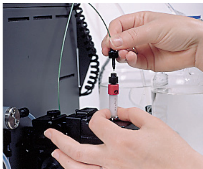
Connecting the column.
