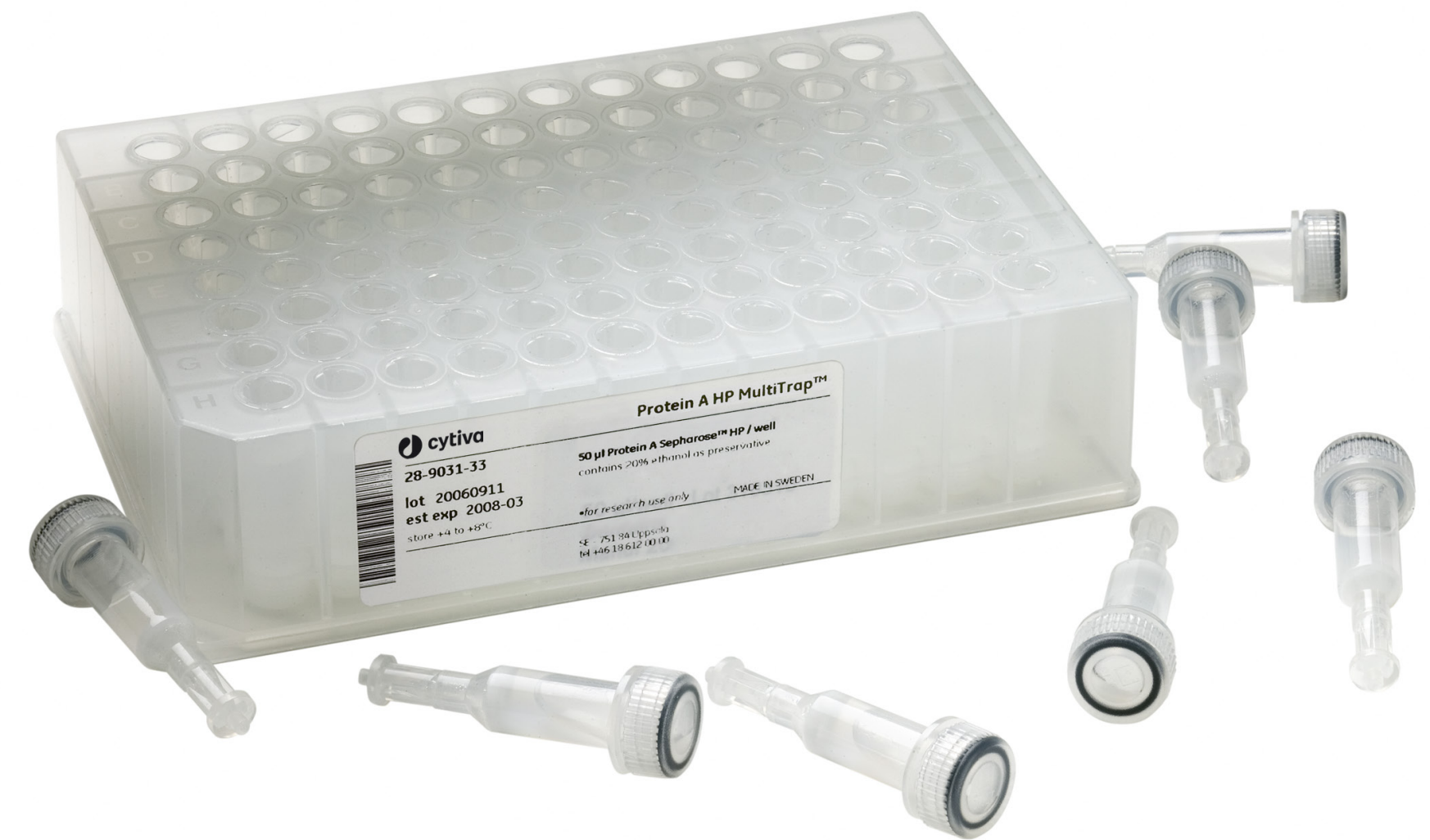
Fig A3.3. Protein A HP SpinTrap spin columns and Protein A HP MultiTrap 96-well plates for the enrichment of proteins from a variety of biological samples.
