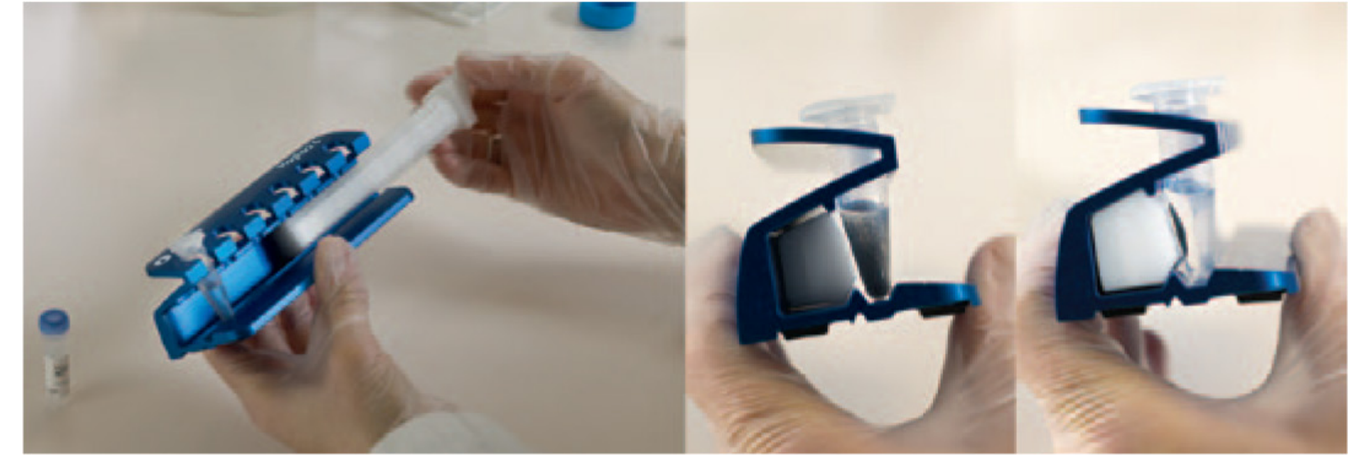
Fig 3.27. The high density of Mag Sepharose beads allows rapid capture by MagRack 6 magnetic device.
