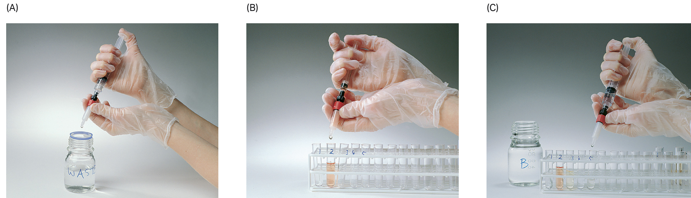
Fig A4.1. Using HiTrap columns with a syringe. (A) Prepare buffers and sample. Remove the column's top cap and twist off the end. (B) Equilibrate the column, load the sample and begin collecting fractions. (C) Wash and elute, continuing to collect fractions.
