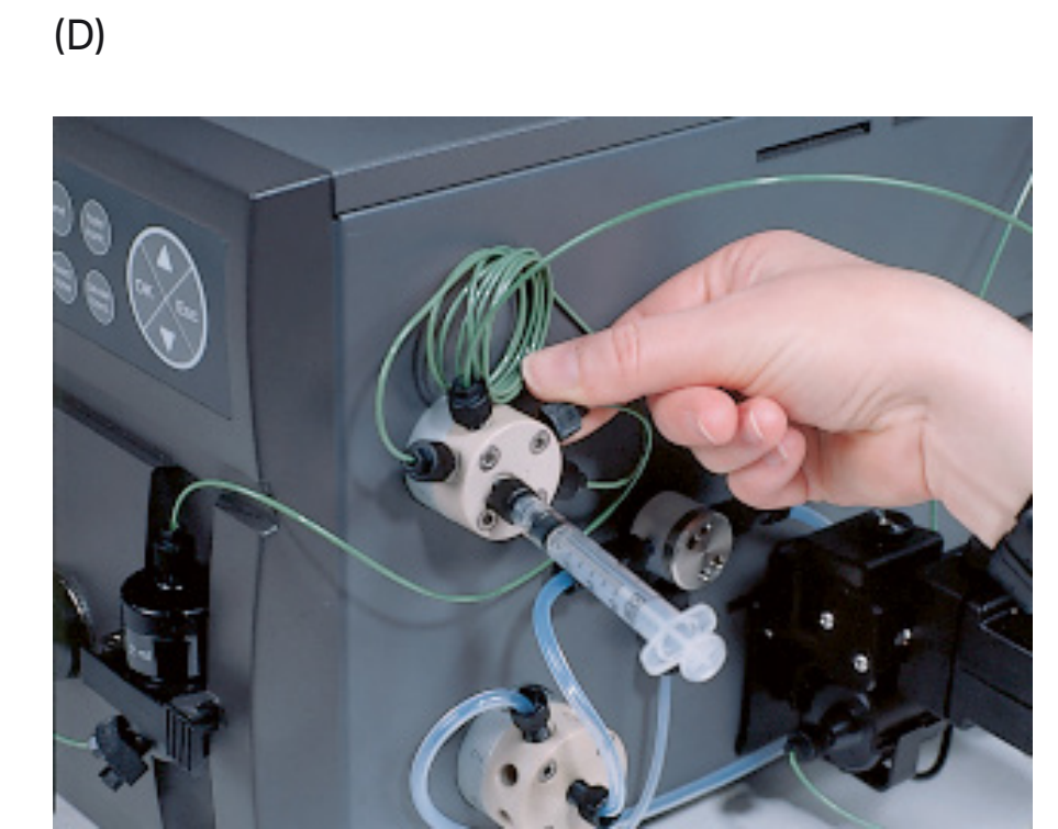
Fig A4.2. Typical procedures using ÄKTAprime plus. (A) Prepare the buffers. (B) Connect the column. (C) Prepare the fraction collector. (D) Load the sample.
