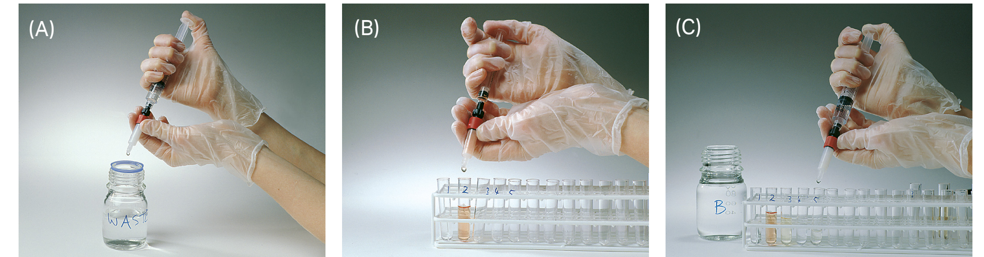
Fig 5.9. Using a GSTrap column with a syringe. (A) Prepare buffers and sample. Remove the column's top cap and snap off the end. (B) Load the sample and begin collecting fractions. (C) Wash and elute, continuing to collect fractions.
